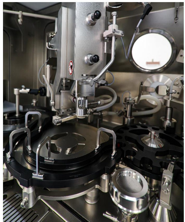
Figure 5: Capping and Crimping Isolator Chamber
